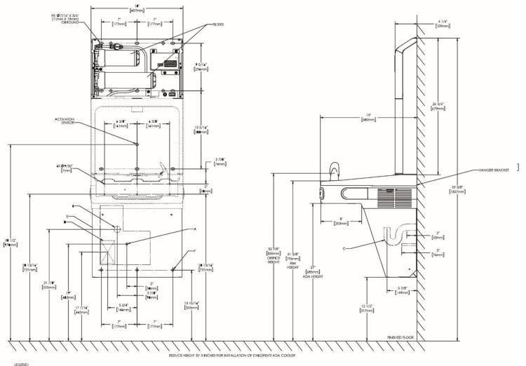
A = Recommended Water Supply location. Shul-off Valve (nof fumished) to accept 3/8" O.D. unalated copper tube. Up to 3" (74mm) maximum out from wall b = Recommended Water Outle location. To accommodate 1-1/4" nominal drain. Drain stub 2" (51mm) out from wall. C = 1-1/4" frag (nof turnished). D = Bechrical Suppov (3) Wite Recessed Duplex Outlet.
