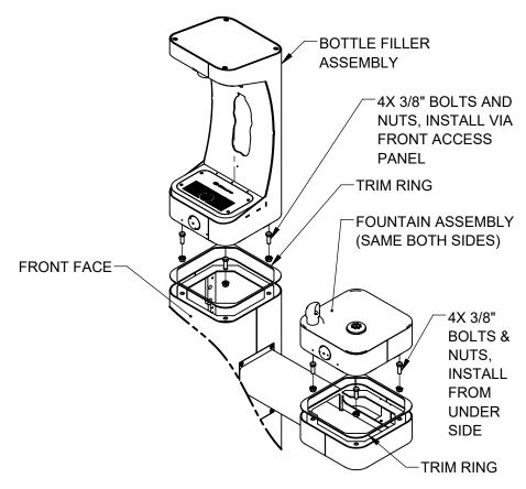
PLACE SQUARE TRIM RING ON BOTTOM OF BOTTLE FILLER AND PLACE BOTTLE FILLER ON TOP OF PEDESTAL, FACING THE FRONT. USE 3/8" BOLTS AND NUTS VIA THE FRONT ACCESS PANEL TO SECURE BOTTLE FILLER TO PEDESTAL. PLACE TRIM RING AND INSTALL FOUNTAINS ON ARMS AS SHOWN. CAREFULLY CENTER BOTTLE FILLER, FOUNTAIN, AND TRIM RINGS, THEN TORQUE BOLTS/NUTS TO 18 FT-LBS
